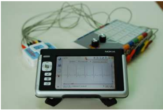
Figure 40. The Nokia770-based mobile ECG application.
