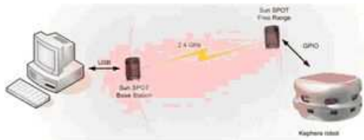
Figure 3. Remote control system.
