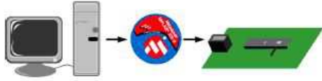
Figure 9. The entire development system with PC host and Trainer board connecting through Microchips in-circuit debugger ICD2 [7].
